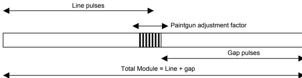
Changing the adjustment factor adds/subtracts pulses to/from the line of a line+gap module. It does not change the overall length of the module. Provided the system calibration is known the length of a pulse can be calculated. For example: where the calibration is 200pulses/metre, each pulse is 5mm long.
