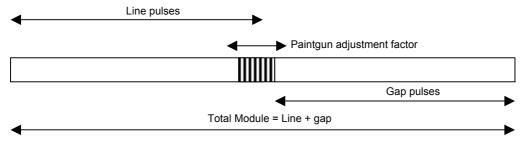
Changing the adjustment factor adds/subtracts pulses to/from the line of a line+gap module. It does not change the overall length of the module. Provided the system calibration is known the length of a pulse can be calculated. For example: where the calibration is 200pulses/metre, each pulse is 5mm long.
